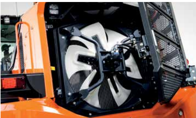
Intelligent fan operation system prevents radiators clogging.
