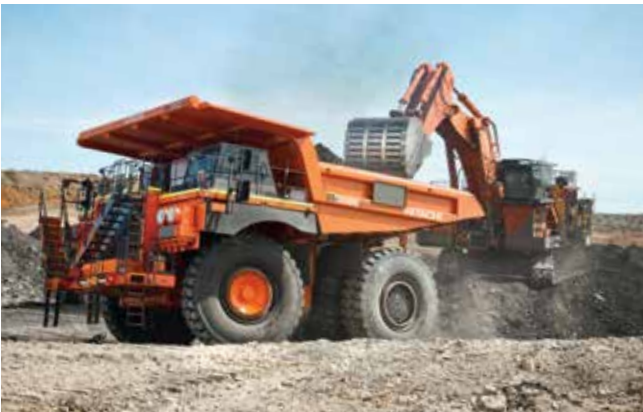
EH dump trucks and EX ultra-large excavators
