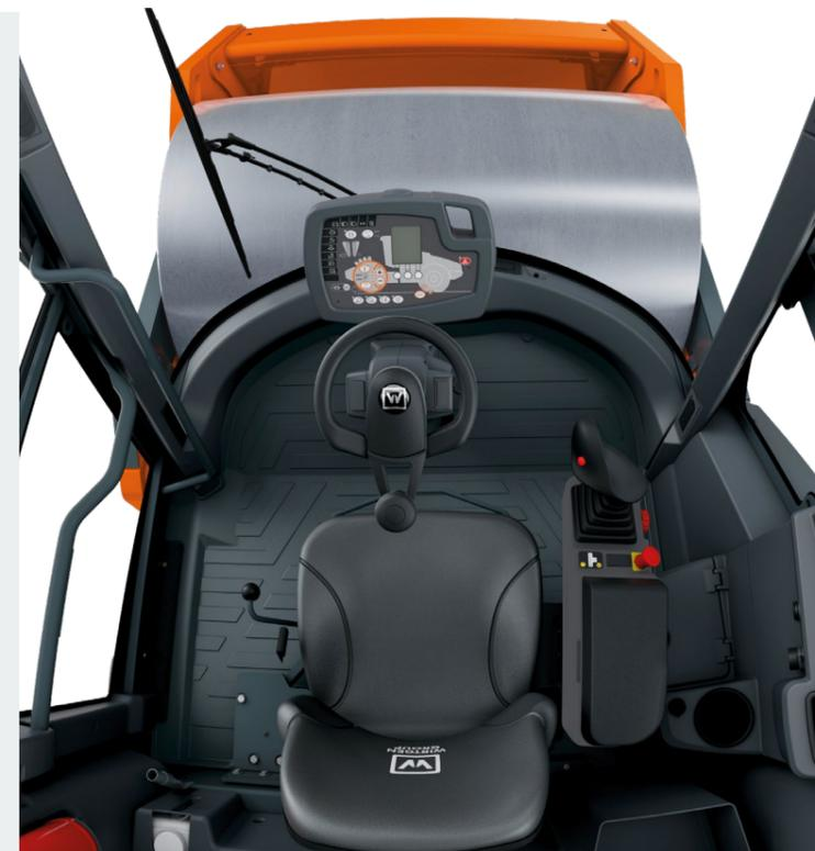
The dashboard behind the steering wheel contains status and parameter displays as well as infrequently used buttons. All displays and switches are grouped into functional units with colour markings. This makes operation easier, since the same applies here as it does to all other HAMM rollers: Same colour - same functional group.
